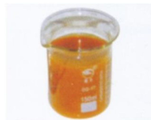
Water draining from untreated inner wall of air compressor.
